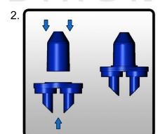
Wearing disposable gloves, snap the mouthpiece securely inside the large ring on top of the base. Label collection tubes as required with sample ID information.
