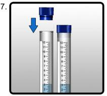
Firmly insert a blue tube cap into each Collection Tube for storage or transportation. Discard the UltraSal-2™ mouthpiece and base in an appropriate manner.
