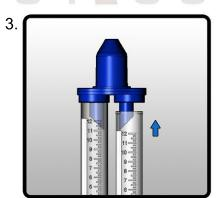
Attach the two Collection Tubes to the bottom of the UltraSal-2™ base by sliding one tube over each outlet and pushing them firmly into the bottom of the base until they snap securely in place.
