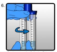
Gently remove the Collection Tubes by holding the UltraSal-2<sup>™</sup> base in one hand, grasping a tube in the second hand, and twisting the tube gently from side to side until the tube separates from the base.
