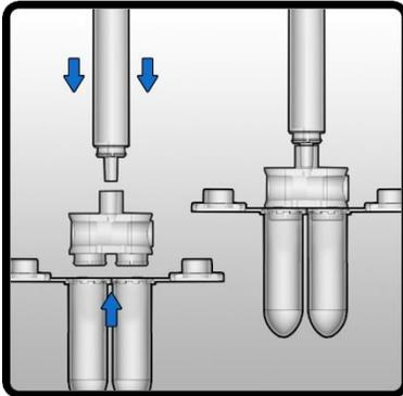
Attach the two Collection Tubes provided to the base of the Universal Filtration and Splitting Unit (“Splitting Unit”) as shown in Figure 2. Attach the Compression Tube into the top end of the Splitting Unit firmly (Figure 2). Sample collection may now begin. Pool saliva in the mouth as you prepare to take the sample.
