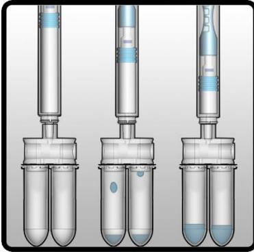
Remove the RNAPro•SAL™ device from the mouth and place the white absorbent pad end into the Compression Tube holding the RNAPro•SAL™ in an upright and vertical position and firmly push the plunger downwards to transfer saliva from the absorbent pad into the Cryofuge tubes. Push and hold for 30 seconds. Note: An optional Tube Rack (Catalog Number TRAC-001) from Oasis Diagnostics® helps maintain the RNAPro•SAL™ device in an upright position during sample acquisition.
