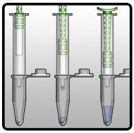
Place the white absorbent pad end into the Plastic Compression Tube holding the Micro•SAL™ device in an upright and vertical position and firmly push the plunger downwards to transfer saliva from the absorbent pad into the Eppendorf Tube. Push and hold for 15 seconds.
