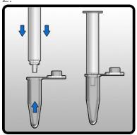
Attach the Eppendorf tube provided to the base of the Plastic Compression Tube firmly.
