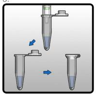
Gently remove the Eppendorf Tube from the end of the Plastic Compression Tube. Add preservative (not provided), if required, and close the lid on the tube tightly.
